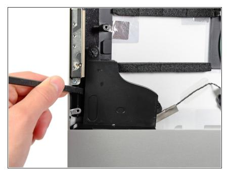
Use the flat end of a spudger to pry the left side of the left speaker away from the side of the outer case.
