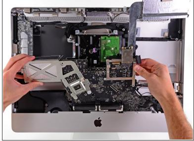
Slightly pull the logic board away from the back of the outer case, then lift it upward to clear the lower front face of the outer case.
