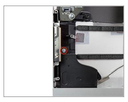
Remove the single 13 mm T10 Torx screw securing the left speaker to the outer case.
