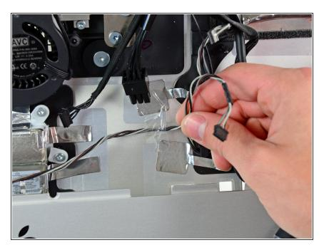
Pull the left speaker cables out from under the strip of tape securing them to the outer case.
