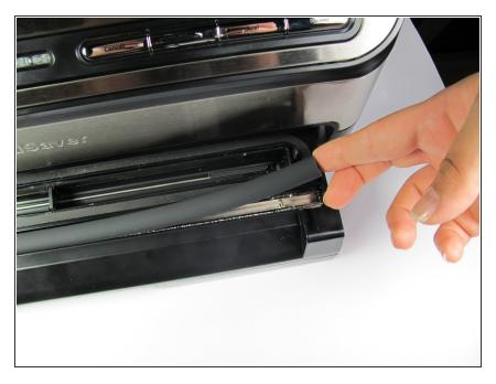
• Gently pull the sides of the rubber seal profile with a finger and remove it from the device.
