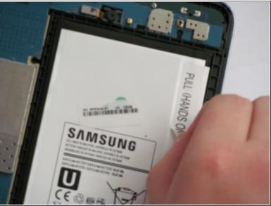
Peel the sticker, reading "PULL (HANDS ONLY)," off of the battery starting at the detachable corner.
