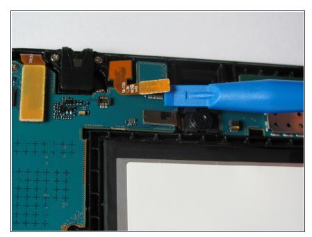
Slightly apply pressure and move the blue plastic opening tool downwards to pop the front camera's gold rectangular connector from its socket on the motherboard.
