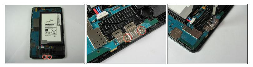
Remove both 2 mm #000 Phillips screws from the metal charger port cover.
