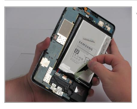
Peel away the green tape starting at the bottom left side.
