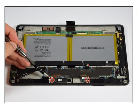
Using a T5 screwdriver remove the two 2.5 mm T5 screws securing the grey camera housing to the device.
