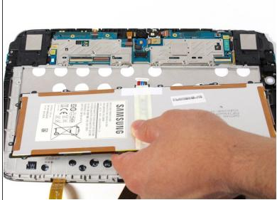
Disconnect the battery by lifting it upward and pulling it away from the connector.
