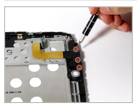
Remove the three 2mm screws along the right side of the device using a PH00 screwdriver.
