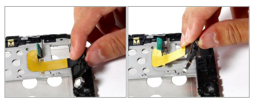
Gently pull battery-audio jack-USB assembly upward, detaching it from its adhesive.
