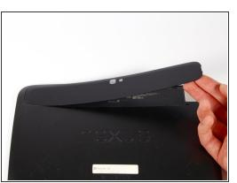
• Using a plastic opening tool, remove the thin plastic cover from back of the tablet by prying up from its small tab.
