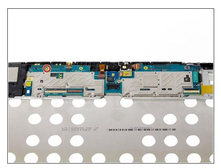
Remove one screw on the logic board with a PH00 screwdriver.
