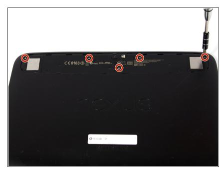
Remove the five 2mm screws on the back of the device using a PH00 screwdriver.
