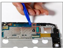
Disconnect connectors around the perimeter of the motherboard.
