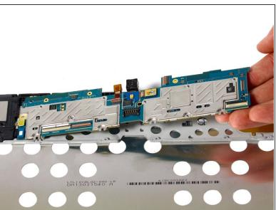
Remove motherboard by gently pulling upward under its corner.
