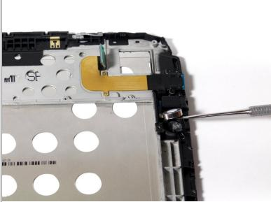
• Unseat the small vibrator motor by gently applying upward pressure with a spudger.
