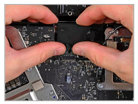
Use your thumbnails on both sides of the Bluetooth/ambient light sensor/camera/left temperature connector to push it toward the top edge of the iMac and out of its socket on the logic board.
