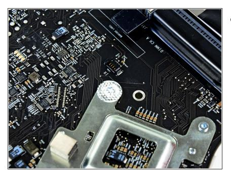
If present, remove the "Warranty void if removed" sticker covering one hidden screw on the heat sink.
