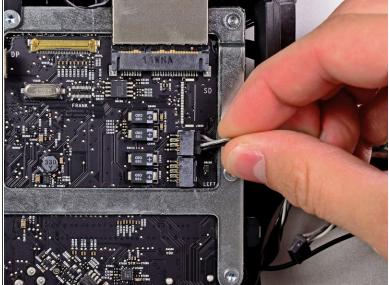
• Disconnect the left speaker and right speaker cables by pulling their connectors toward the right side of the iMac.
