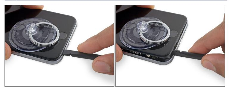
Twist the spudger to widen the gap between the front panel assembly and the rest of the phone.
