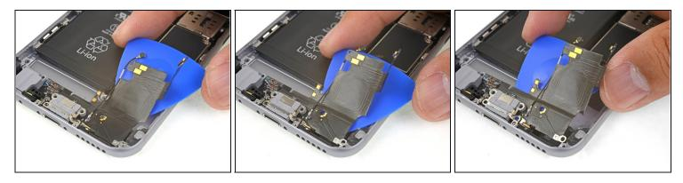
Insert the flat end of a spudger between the Lightning connector assembly and rear case to break up the remaining adhesive.
