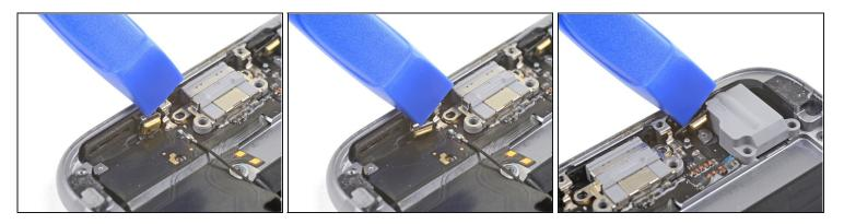
• Use an opening tool to separate the microphones from the bottom edge of the rear case.
