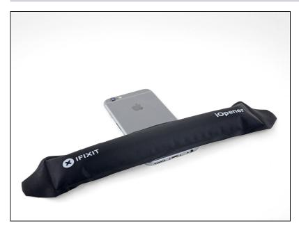
Heat an iOpener and apply it to the back of the phone near the bottom edge for one minute.
