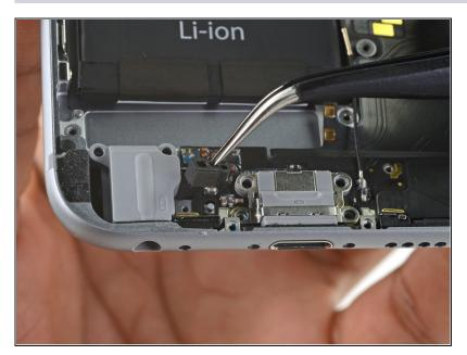
Remove the plastic microphone bracket.
