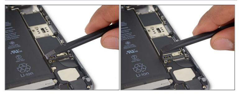
• Push the battery connector away from the logic board until it stays separated from its socket, so as to avoid any accidental connection to the battery while you work.
