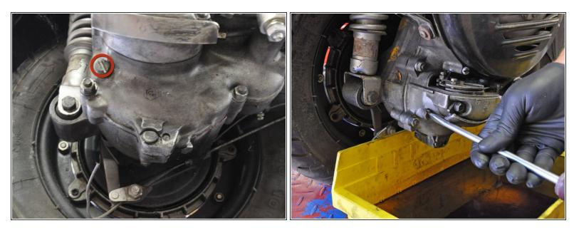
Use a large flathead screwdriver to remove the oil fill plug.
