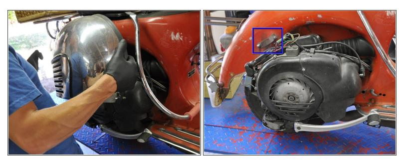
Carefully lift the engine cover up and away from the scooter, mindful of the mounting bracket near the rear of the engine.
