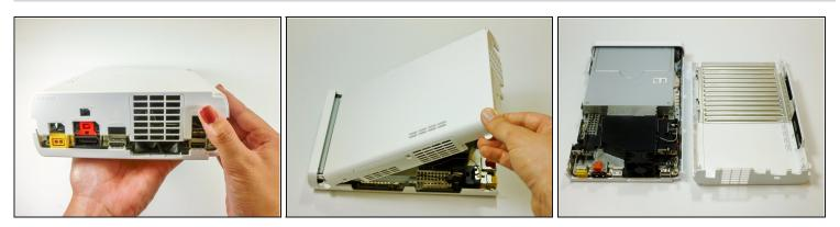
• On the back of the console, lift up and release the main top cover.
