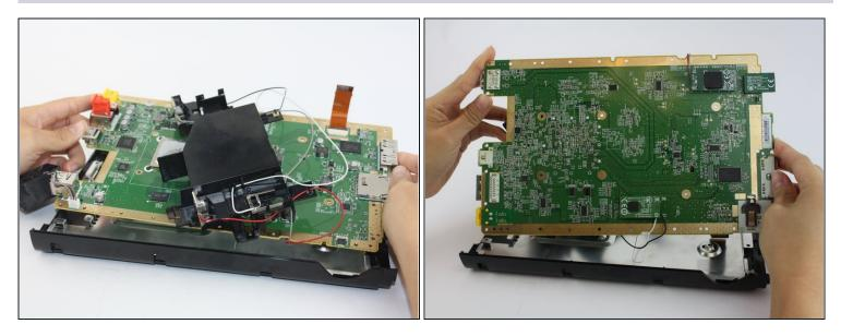
• At this point, the motherboard should easily separate from the lower tray.
