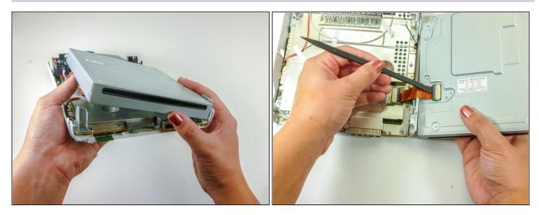
• Rotate the device so that the disc drive slot is visible.
