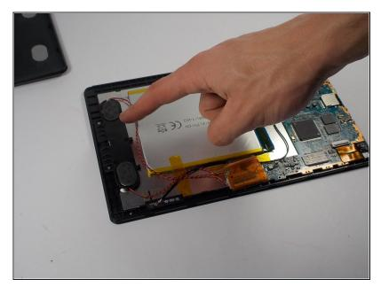
The external speakers are located in the black plastic fixture near the battery as pointed to in the image.
