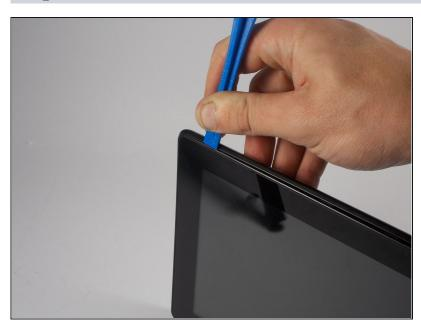
Take the plastic opening tool and insert it into the crease between the screen and the plastic casing and press down.
