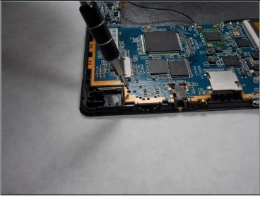
• Use a J0 sized Phillips head screwdriver to remove the three 3.175mm long Phillips head screws from the motherboard.
