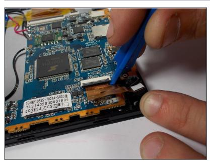
Use a smaller plastic opening tool to lift up the ZIF connector in which the cameras are plugged into.
