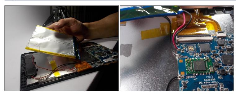
• Lift up the battery it will be glued to the device.
