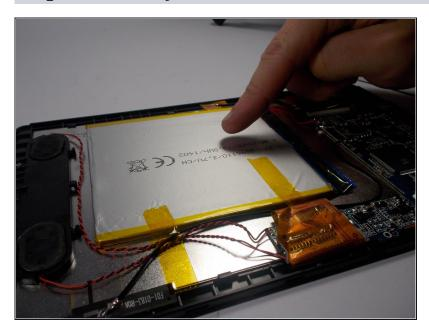
The battery is the bigger square object in the center of the device held down by 3 pieces of yellow tape.
