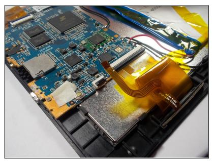
• Then remove the ribbon cable from the ZIF connector.
