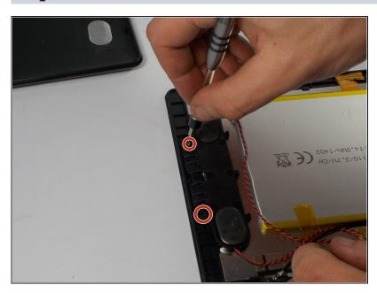
Use a J0 sized Phillips head screwdriver to remove the two 3.175mm long Phillips head screws from the speaker fixture.
