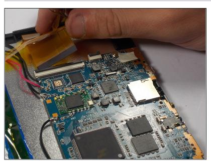
Remove the ribbon cable from the ZIF connector, it is next to the volume buttons.
