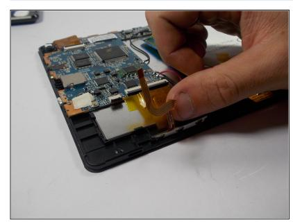
⚠ Make sure to separate the volume button's cable from the cable connecting the motherboard to the screen
