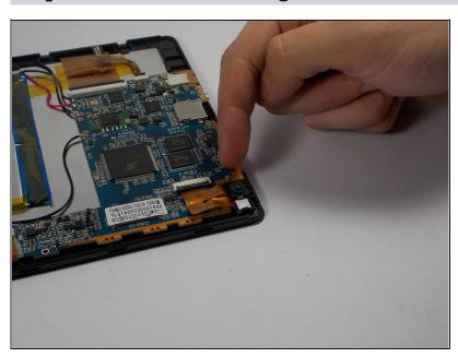
The front/rear facing cameras are located in the corner of the device one is facing toward you and is black. The other is facing away so you will see the white backing.
