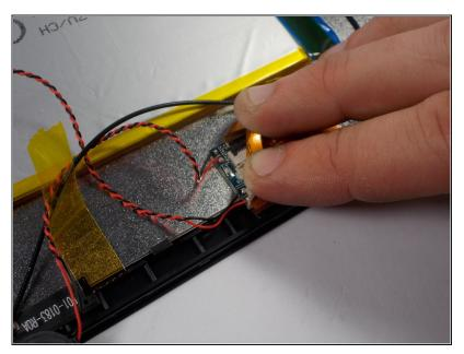
The two wires that connect the speakers to the motherboard must be removed next. In order to replace the speakers you will need to solder them back into place.
