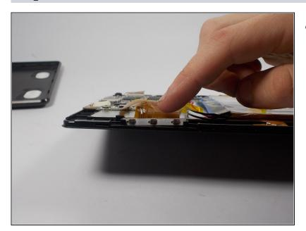
You can locate the volume buttons on one of the longer sides of the tablet.
