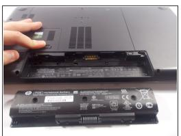
Press and hold the release switch, and then slide the battery out. Insert the new battery into the slot and you're done!
