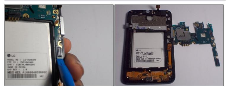
• Push the blue lifting tool up underneath the logic board and pull it upwards removing it from the device.
