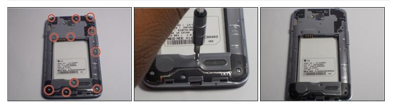
• Remove the eleven 4mm screws using a Philips head screw driver.
