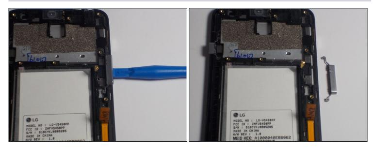
• With the device facing up lift with your fingers or the blue lifting tool to remove the volume buttons from the device.
