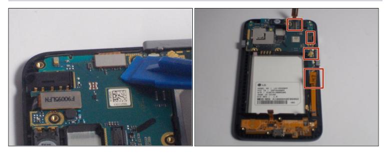
• Disconnect the remaining ribbon plugs and connectors. (Only remove the highlighted cables for the removal of the logic board.)
