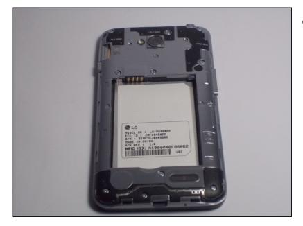
• Push on the top of the battery downward and pull the battery off of the device.
