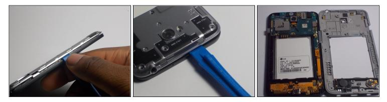
• Insert the plastic opening tool into the side of the device and pry off silver covering. Push up against the back covering when the tool is inserted to detach from the phone.
