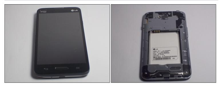
• Flip the device over and remove the back covering.
