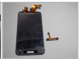
Using tweezers lift the home button to remove the home button from the device.
