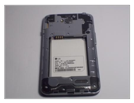
Push on the top of the battery downward and pull the battery off of the device.
