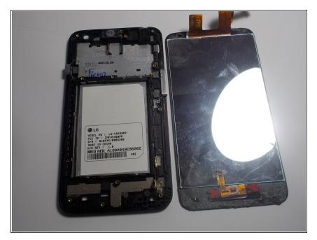
Pull the screen off of the body of the device. (Mind the circuits when removing the screen. The home button is likely to fall off.)
