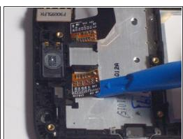
Using the blue lifting tool carefully remove the screens connectors.
