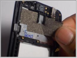
Using a prying tool, carefully remove the silver/ black tape used to hide the screens connectors.
