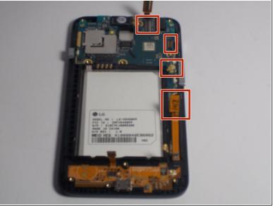
Disconnect the remaining ribbon plugs and connectors. (Only remove the highlighted cables for the removal of the logic board.)
