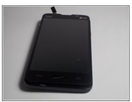
Flip the device so the screen faces you. Using a prying tool, at the corners on the screen begin to pry off the screen. (It will sound like tape being removed.) Avoid scratching the device with the prying tool.
