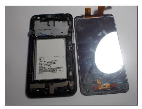
Pull the screen off of the body of the device. (Mind the circuits when removing the screen. The home button is likely to fall off.)
