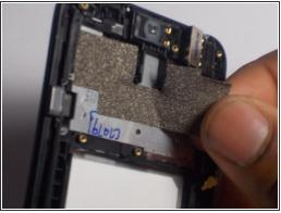
Using a prying tool, carefully remove the silver/ black tape used to hide the screens connectors.
