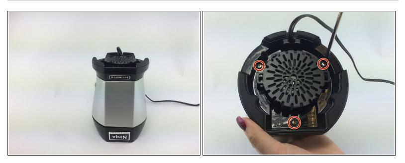
Turn the blender over and unscrew the three 14 mm screws holding the slotted base in place.
