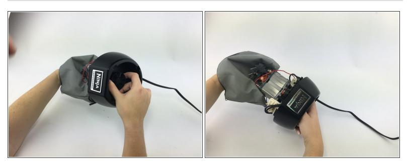
Untwist the small rubber connector to detach the plastic from the motor.
