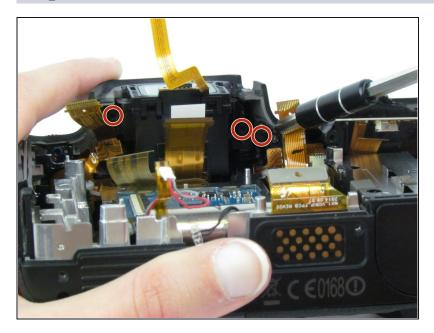
• Use the Phillips #00 screwdriver to remove the three black 3.8 mm screws below the viewfinder.
