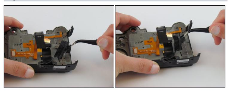
• Use <u>tweezers</u> to remove the glued rubber piece.
