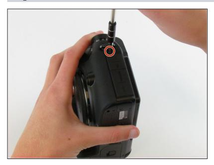
• Use the Phillips #00 screwdriver to remove one 5.5 mm screw on the left, above the HDMI port.
