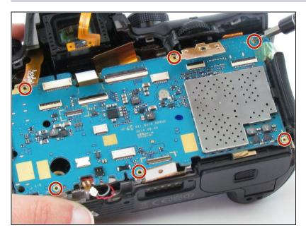
• Use the Phillips #00 screwdriver to remove the six silver 4.5 mm screws.
