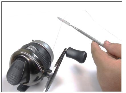
• Cut the line free from the Zebco 33 spool. Pull the line through the front spool cover and then through the line.
