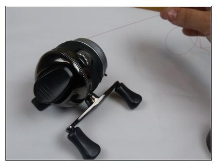
Remove the old line remaining on the Zebco 33 by pressing down on the large spool release button on the back of the reel. Pull the old line off the reel.
