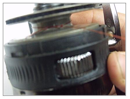
Attach the line to the spool of the Zebco 33 with a knot. Double the knot and then pull the knot down tightly against the spool of the reel. Clip the extra line from the knot.
