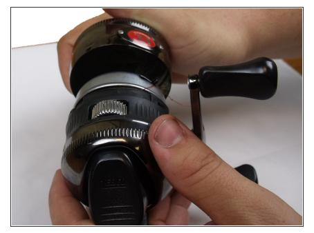
Put the front spool cover back on the reel. Hold the line a few inches in front of the spool and apply slight tension to the line. Wind the line onto the reel by turning the handle of the reel.
