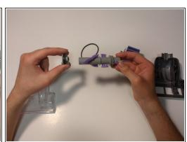
Pull out the side screws from the right and left side of the old roller brush and put them on the replacement roller brush.
