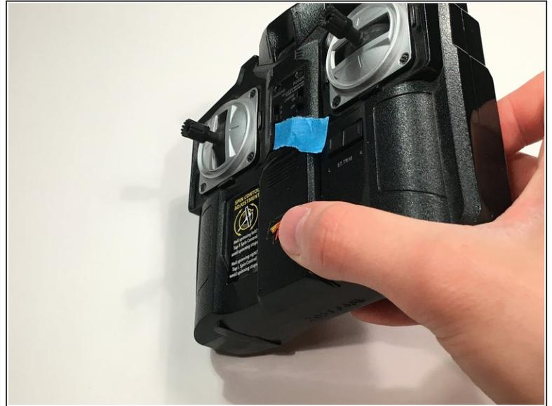
**i** Power off the controller before disassembly.
