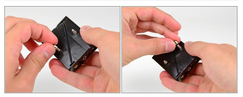
• Use your free hand to place the two metal spacers over the screw threads (one per screw).
