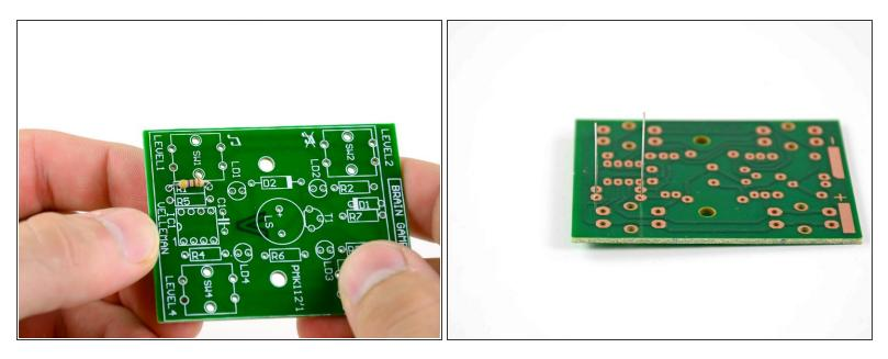
Place the leads of the resistor through the holes on either side of the rectangle marked R1 on the circuit board.
