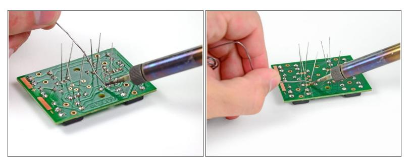
• Solder each of the LEDs to the circuit board and cut the excess off each lead.
