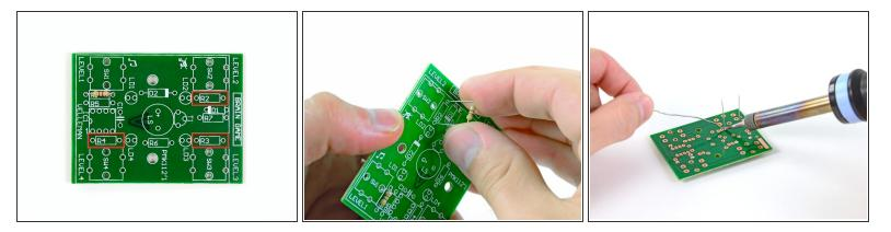
Install the three remaining 470 Ω resistors (yellow/violet/brown) into the terminals marked R2, R3, and R4.
