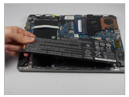
Carefully use light upward pressure to unseat the battery from the case, but do not pull on the cord or try and completely remove the battery from the case.
