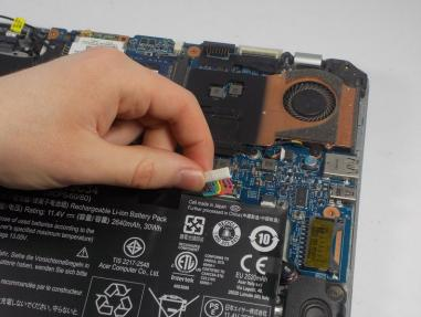
• Finally, disconnect the battery from the motherboard by undoing the power connector. To undo the connector, simply apply light to moderate pull on the sides of the connector.
