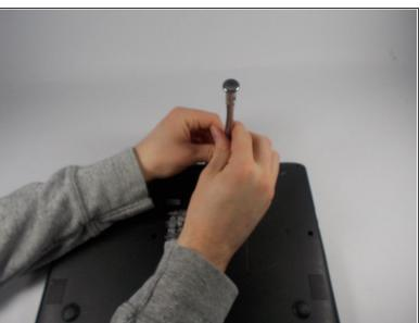
• Towards the top right corner of the laptop, there is a rubber piece covering the final screw holding the cover on, as well as a set of pins. Use your fingernail to remove this piece of rubber, and then unscrew the hidden 5mm screw.
