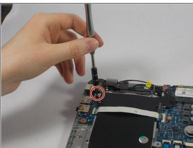
Remove the the two screws that hold the hard drive tray in place.
