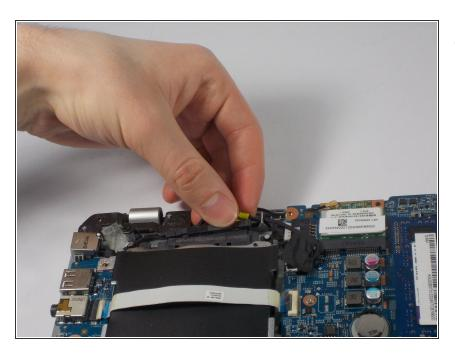
Remove the SATA cable that is attached to the top of the hard drive.
