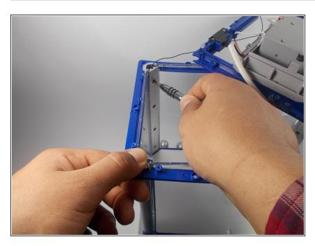
Loosen all eight screws using your phillips head #1 screwdriver so that the glass can be removed.
