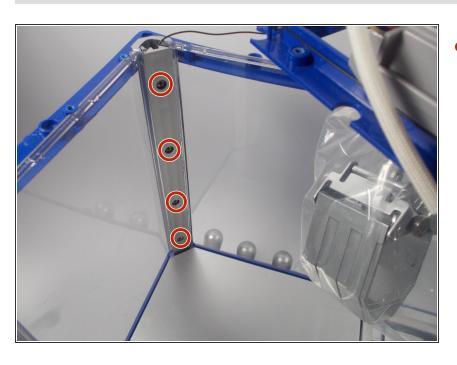
The glass you intend to replace will have four 6mm #1 phillips head screws on either side located in the silver corner pieces.
