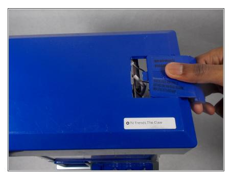
Place thumb on grip section and pull away from the Claw machine.
