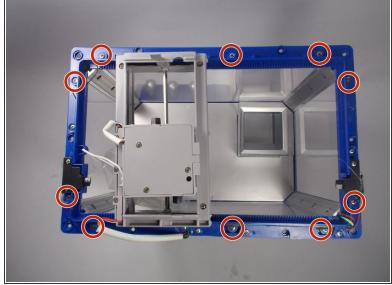
• Remove the ten 6 mm phillips #1 screws from the top flange.
