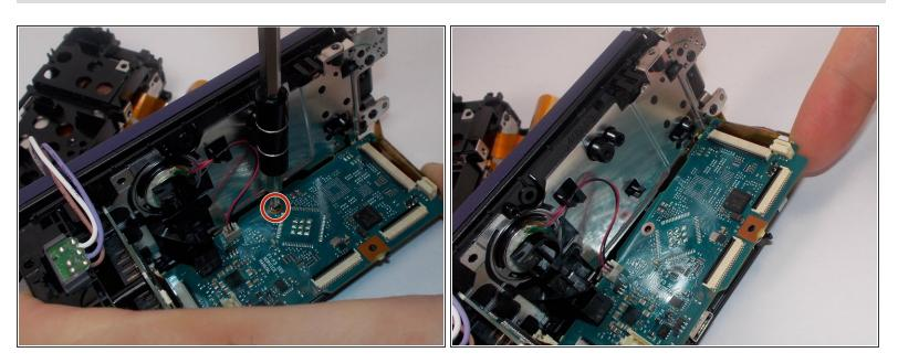
Use the Phillips #0 screwdriver to remove the 4mm screw shown.
