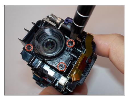
Remove the 3 (4mm) screws on the front of the lens using the Philips #0 Screwdriver.
