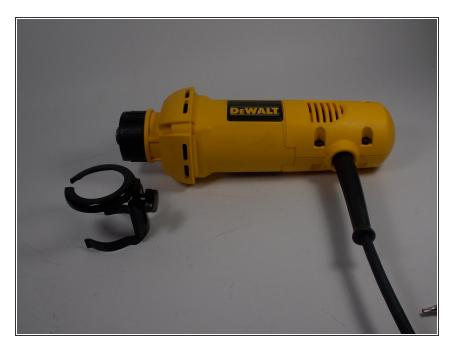
Remove the depth guide from the top of the tool.
