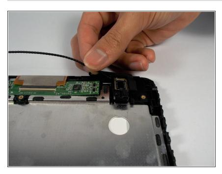
Once the screws are removed, lift up on the speakers to remove them from the case.
