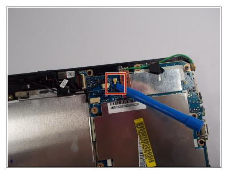
Using the plastic opening tool unplug the black cable by placing the tool under where the cable meets the plug and lift up.
