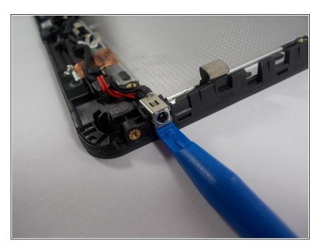
Using the plastic opening tool gently lift up the charging component out of its slot in the case.
