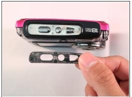
Insert the flat end of wide metal spudger into the seam of the plastic buffer surrounding the buttons and pry it open.
