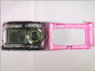
Wedge your fingers in the opening and slowly pull the front casing away from the bottom casing until it complete separates from the device.
