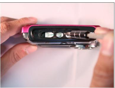
Apply pressure and turn counterclockwise to remove the indicated 2.5 mm screw.
