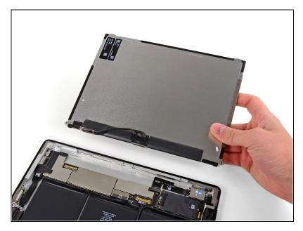
Remove the LCD assembly from the rear panel assembly.
