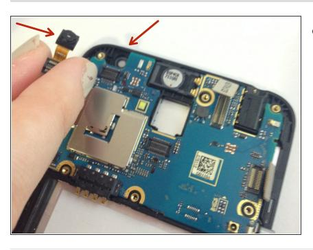
After removing this ribbon cable, you will be able to easily remove the front facing camera with your fingers.
