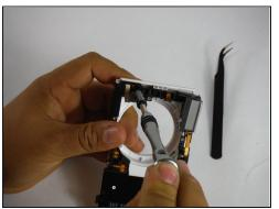
• Using the iFIXIT curved nose <u>tweezers</u>, gently remove the ribbon cable for the flash. Doing so will reveal yet another hidden screw. Remove this with the iFIXIT screwdriver and PH00 bit to release the flash assembly.
