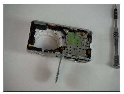
Having completed the previous guides up to this point you should be left with the chassis and internal frame exposed
