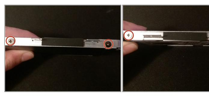
Remove the 4 screws holding the hard drive in the caddy. There are two screws on each side.
