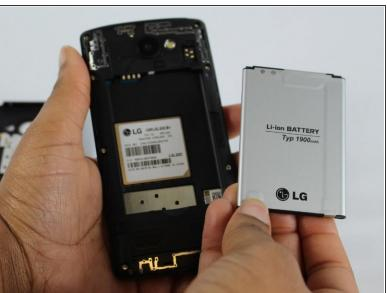
Use the thumb tab to remove the battery.
