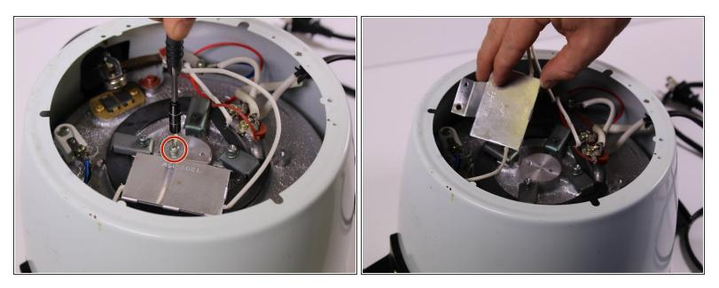
• Remove the 6mm Phillips screw that holds the stainless plate.
