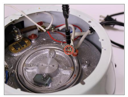
• Remove the 7mm Phillips screw that holds the white & maroon wires connected to the heating element.
