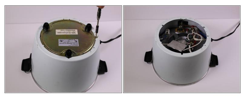
• Remove the one 7 mm Phillips screw from the side of the brass panel.
