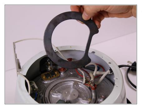
Using your hands, remove the heating plate that is on top of heating element.
