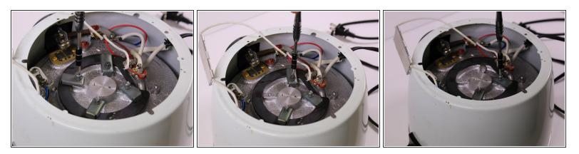
Remove all four of the 15mm Phillips screws from all four of the brackets that hold the heating element in place
