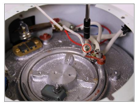
Remove the 7mm Phillips screw that holds the white wire connected to the heating element.
