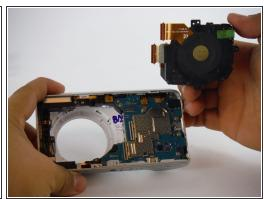
Now that the screws and ribbon cables have been removed, gently pull the lens assembly up from the the camera and remove it.
