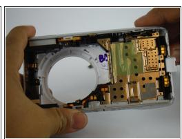
Now, remove the motherboard completely from the chassis.
