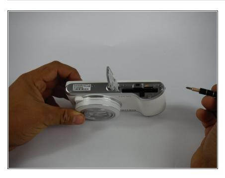
Use the screwdriver to remove screws listed in step 2. There are a total of six 4mm screws.
