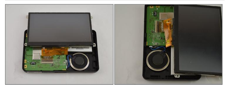
• Carefully move the display out of the way of the speaker revealing the blue and black cord from the speaker.
