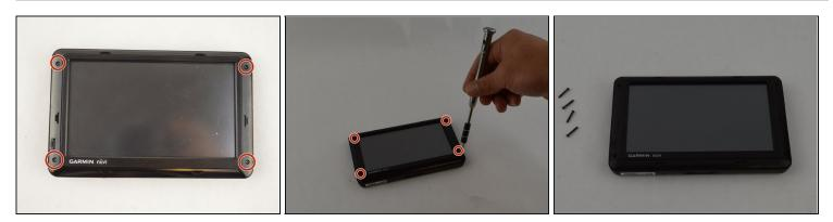
• Remove the four 11.0 mm screws using the Torx T5 screwdriver.
