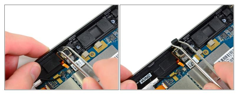
• Use your tweezers to remove the black rubber grommet between the microphone and rear case.
