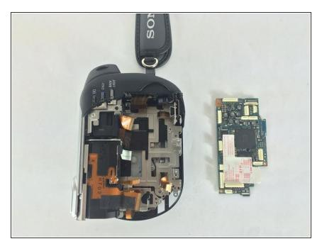
• Lift the motherboard up from the outside edges to remove.
