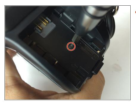
Remove the 2mm #0 Phillips screw behind the battery.
