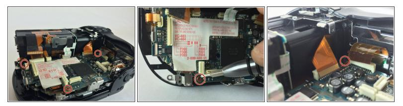
Remove 3 brown copper screws. Each copper screw has a #0 Phillips head and is 2.8mm in length.
