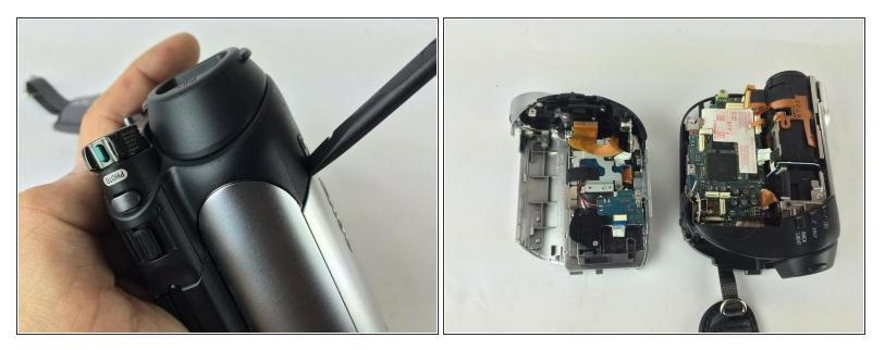
• Once all the screws are removed you can safely pry open the camera case using a spudger.
