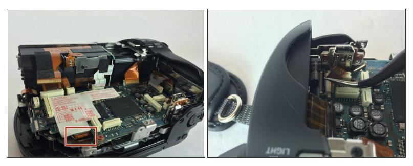
Remove all ribbon connectors from the motherboard using tweezers. Simply grab each ribbon cable and pull straight out of the connector.
