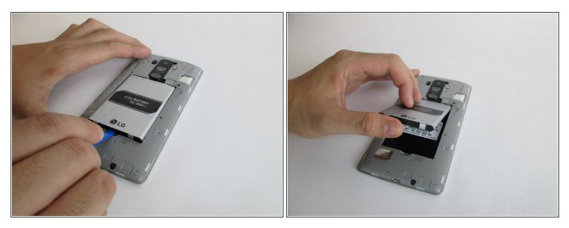
Insert the plastic opening tool into the indent at the bottom of the battery and lift up. Fully remove the battery with your fingers.
