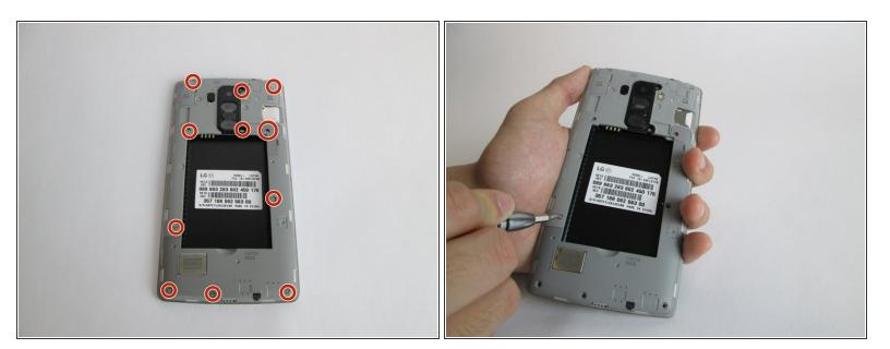
Carefully use the 3.9mm Phillips #00 screwdriver to remove the eleven visible screws found on the back. The screws to be removed are marked with the given indicators.
