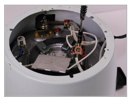
Remove the 10mm Phillips #3 brass screw above the heating element that connects the white power cord wire and the maroon wire.
