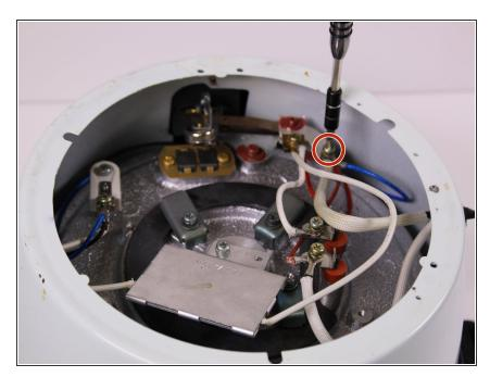
Remove the 7mm Phillips #3 brass screw that connects the white power cord wire and blue wire closest to the power cord.
