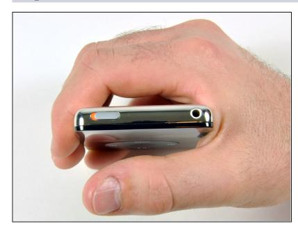
i Before opening your iPod, ensure that the hold switch is in the locked position. The slider should be all the way to the right if your iPod is facing you.
