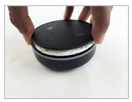
Turn the assembly over and lift up the plate with the buttons.
