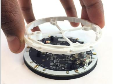
• Turn the plate over, then lift and remove black gear and the white plastic ring.
