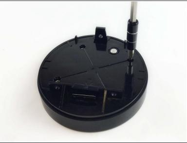
Unscrew the four 9.7 mm T9 torx screws from the bottom of the volume ring assembly.
