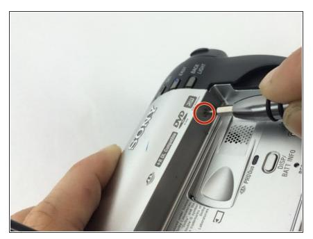
Remove the 5mm #0 Phillips screws on the underside of the LCD tuck-away.
