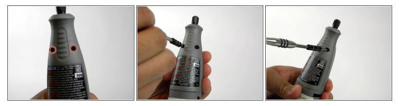
• Remove the two screws from the back of the device with the TR10 Torx Security screwdriver.
