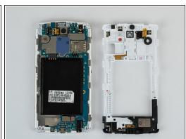
Work a plastic opening tool around the perimeter of the phone to separate the midframe from the rest of the phone.
