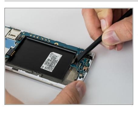
Use the flat edge of a spudger to disconnect the motherboard ribbon connector.
