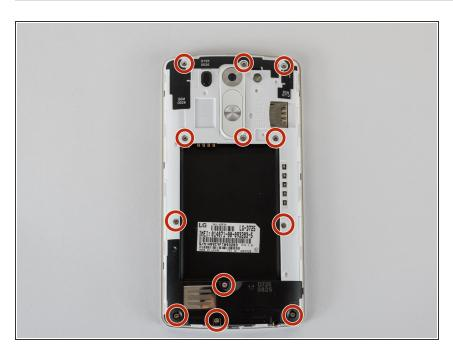
Remove the twelve Phillips #00 screws securing the midframe to the rest of the phone.
