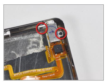
Remove the two black Phillips screws that are securing the headphone jack to the lower casing.
