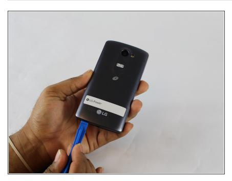
Slide a plastic opening tool between the back and front panel at the bottom.
