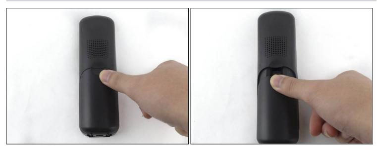
• Find the bump where the battery cover meets the phone. Put your thumb here, and push and slide the cover down.
