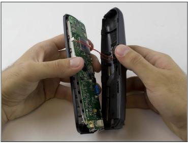
• Use a plastic opening tool to remove the handset case.
