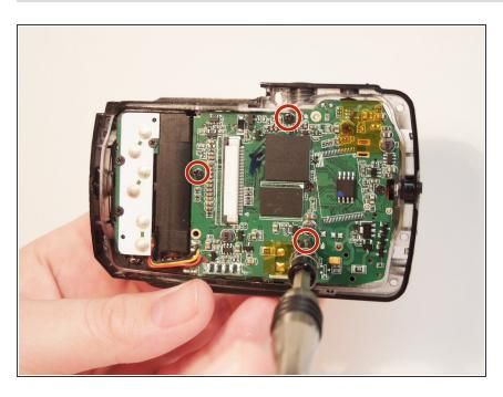
Remove three screws holding the motherboard into the casing using the PH00 bit screwdriver bit
