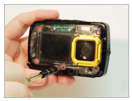
Remove the five silver screws from the inner casing using the PH00 screwdriver bit
